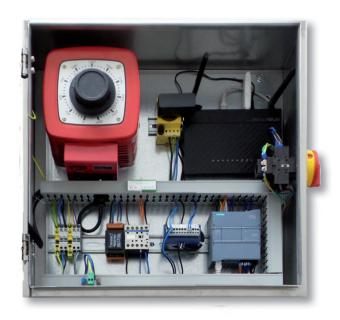
Choose a Universal head stunner by Dutch Vision Solutions, developed for small scale meat processing, compliant with the EU1099 norm.
